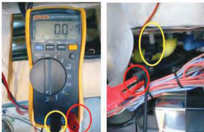
Figure 21 Multimeter connection to the flame control plug
